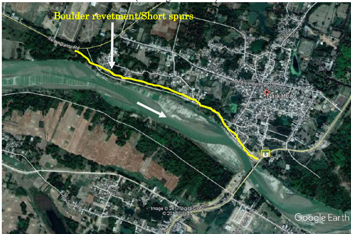
Figure 9.8 Provision of protection to the left embankment upstream of the bridge (SH5) in the form of boulder revetment/short spurs at Rajendra Nagar (Chainage = 251.5 km)
