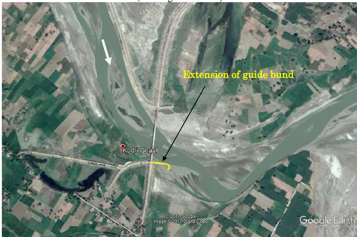
Figure 9.10 Extension of the existing left guide bund of about 90 m downstream at Kodri ghat (chainage 418 km)
