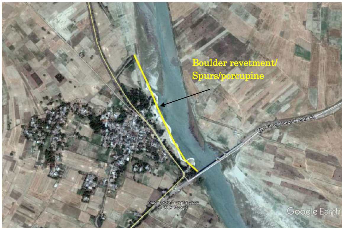
Figure 9.5 Boulder revetment/porcupine/series of spurs on right bank over a length of 700 m upstream of the bridge at Peepeganj (Chainage = 160 km)
