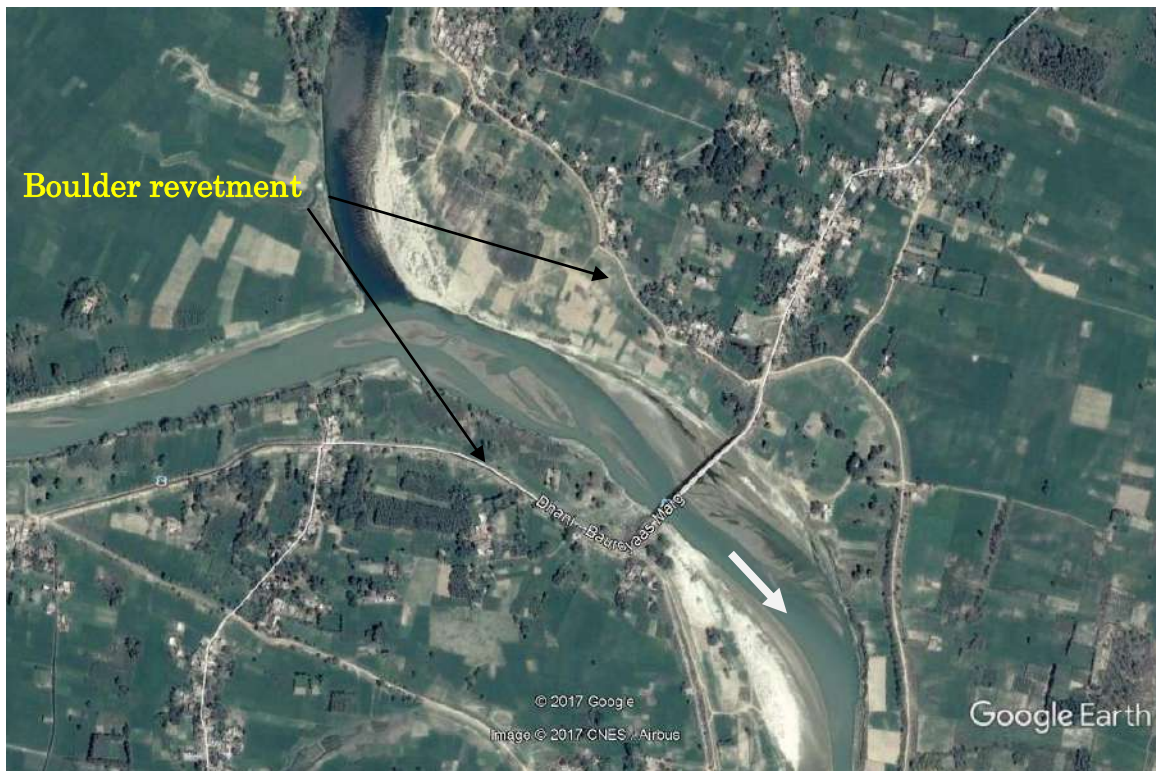
Figure 9.7 Boulder revetment to the existing both sides embankments at Dhani (Chainage = 212 km)
