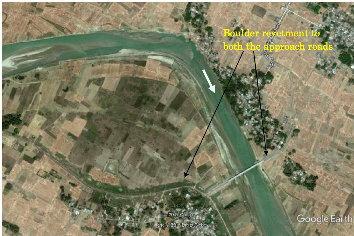
Figure 9.9 Provision of boulder revetment to both the approach roads at Tighra (Chainage 272.5 km )
