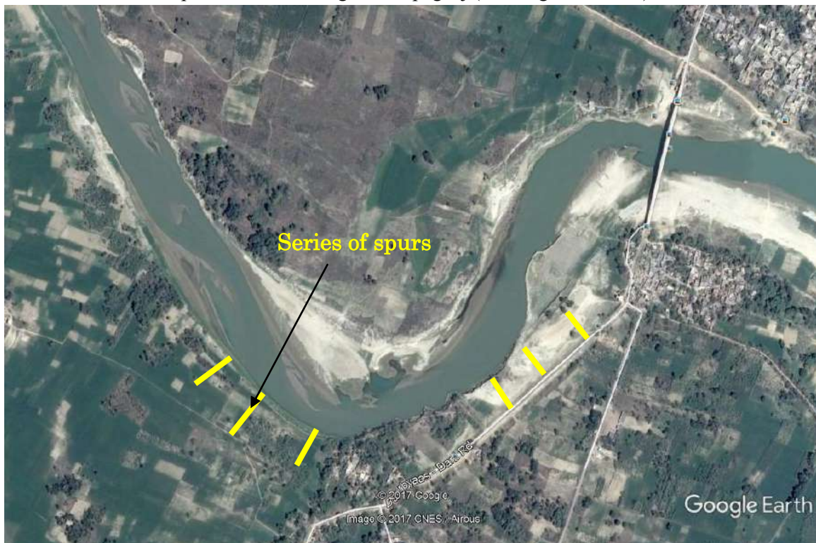
Figure 9.6 Provision of series of spurs towards left side at Dhani (Chainage = 205 km)
