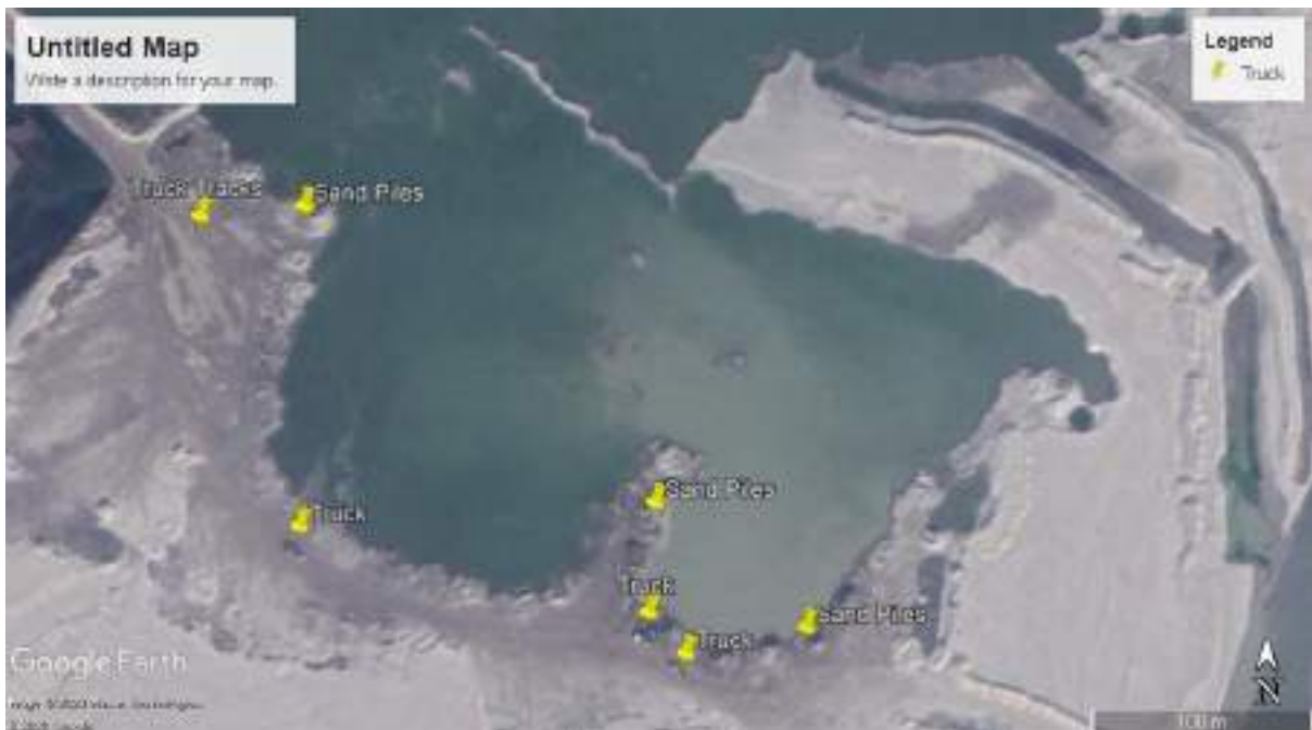
Figure 30(a): Altered Yamuna bed and bank profile as a result of mining of white sands deposits
