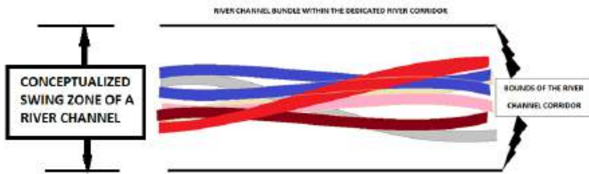
Figure 3: Schematic explaining the concept of alternate flow paths within the dedicated river corridor
