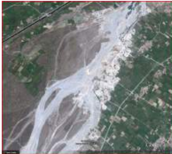
Figure 28: Braided dry river bed sensed on the basis of reflectance of white sands deposits
