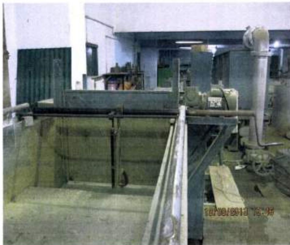
Fig. 3.5 Depth integrated suspended load sampler for the collection of suspended load
