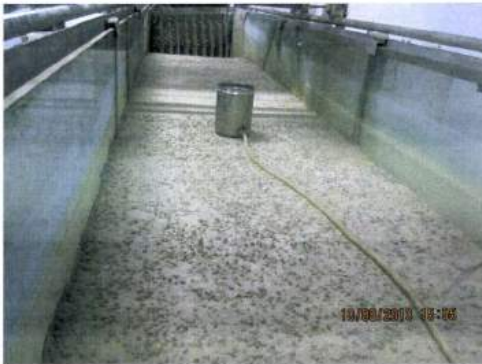
Fig. 3.3 Cylindrical container connected with pipe used for the measurement of bed slope
