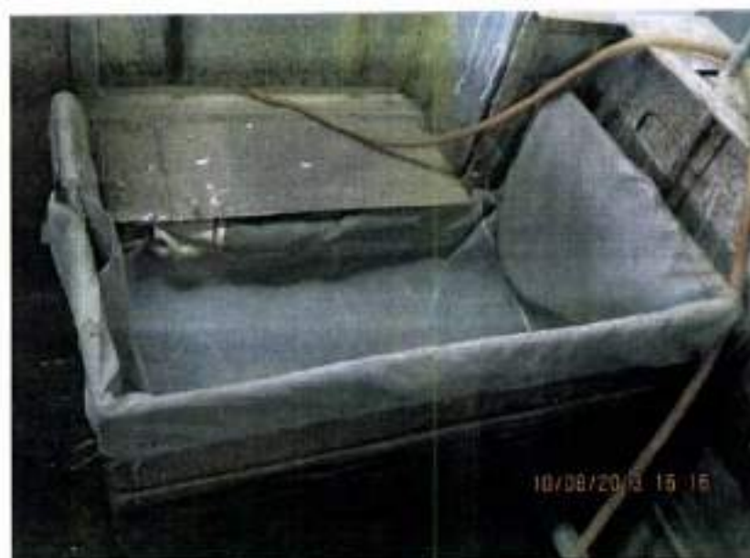
Fig. 3.4 Rectangular trap used for the bed load collection
