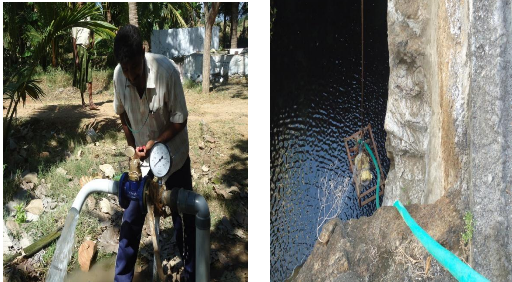
Figure 4.13 Photographs of Pumping test conducted in the field
