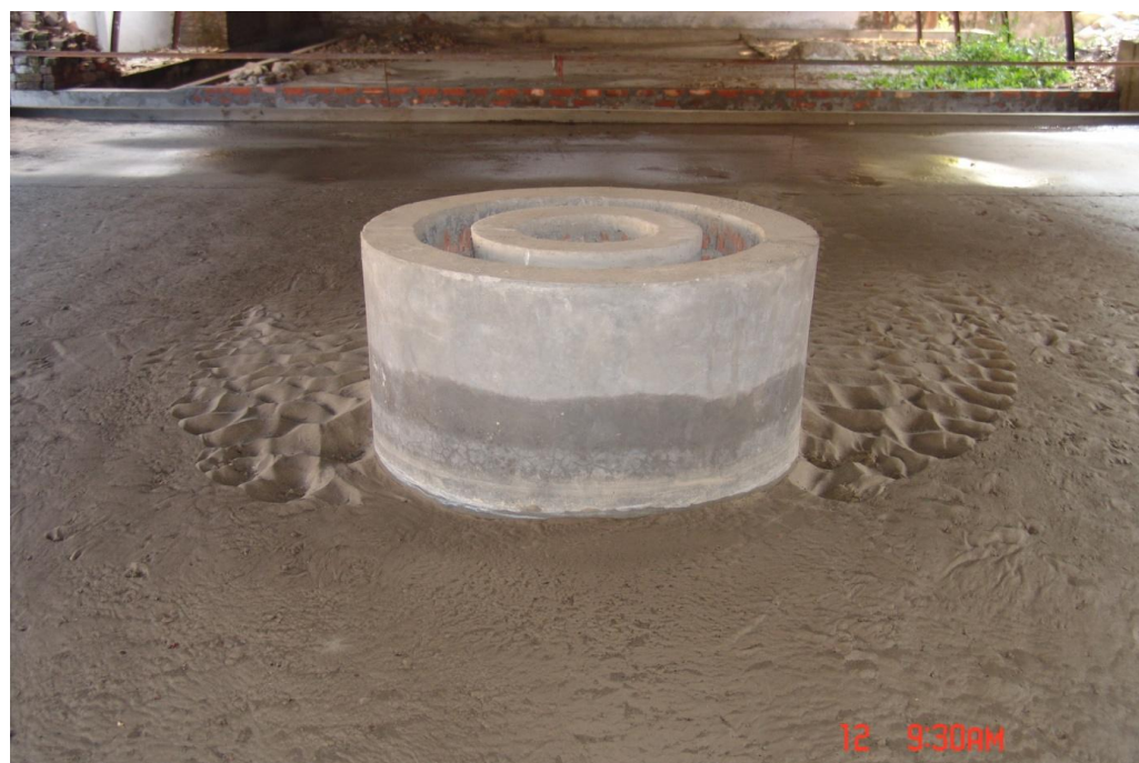
FIG.A8 Scouring around Pier Exposed to Different Flow Conditions
