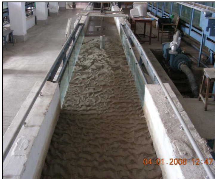
FIG.3.2 Photographic View of the Experimental Flume
