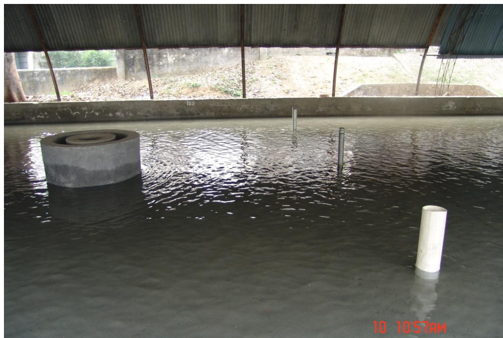
FIG. A6 (a) Piers of Different Sizes Exposed to Different Flow Conditions
