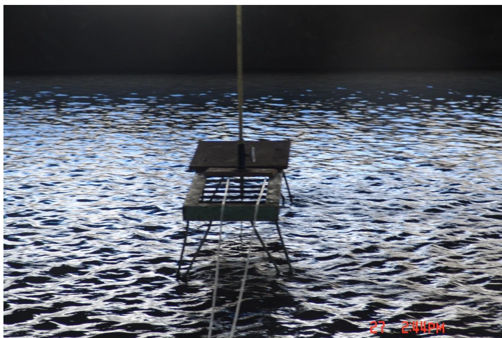
FIG. A4 Flow Measurements using Pitot tube
