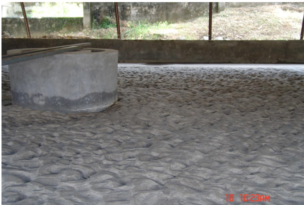
FIG. A7 Scouring around Pier Exposed to Different Flow Conditions
