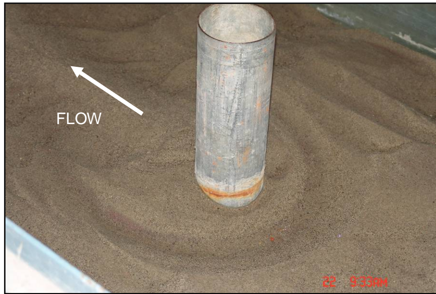
FIG.4.20 Photographic View Showing Geometrical Configuration of Scour Hole without Collar for Live-Bed Condition with Sediment Feed for a Depth of 9.0 cm and u^*/u_{*c}=1.49
