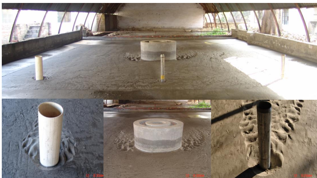
FIG. A9 Piers of Different Sizes Tested for Scouring Under Same Flow Conditions
