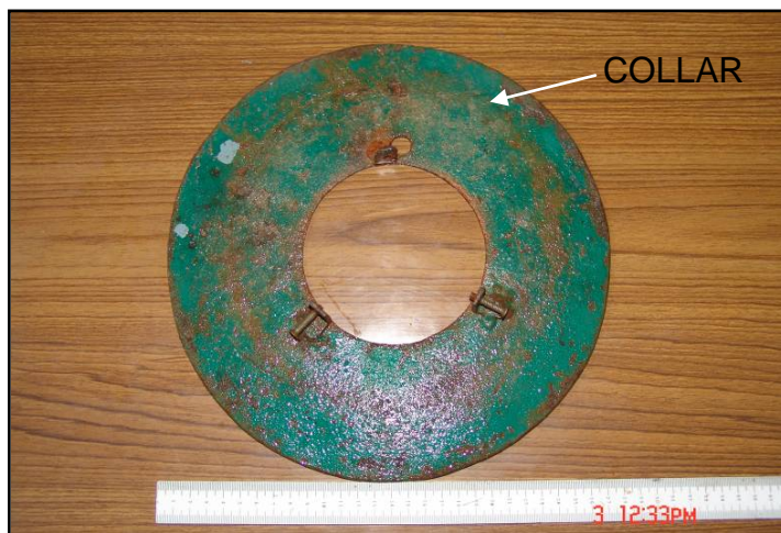
FIG.3.9 Photographic View of Collar Size 2.5b for 0.114 m Pier
