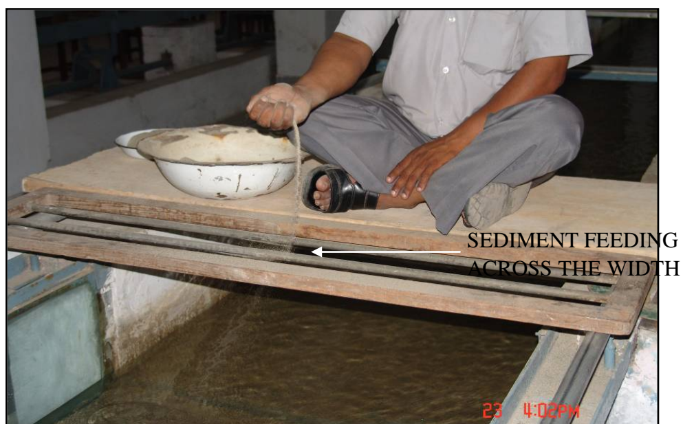
FIG.3.7 Photographic View of Feeding of Sediment
