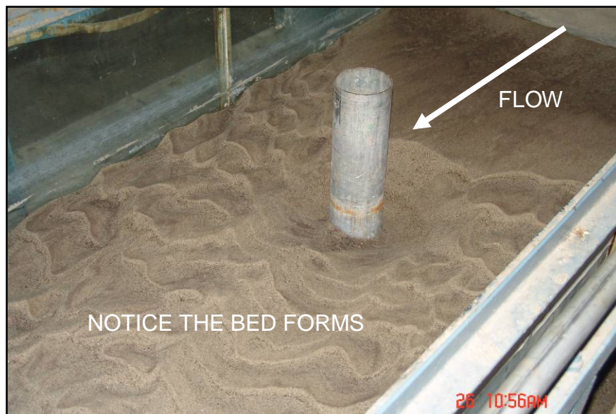
FIG.4.21 Photographic View Showing Geometrical Configuration of Scour Hole without Collar for Live-Bed Condition with Sediment Feed for a Depth of 7.0 cm and u^*/u_{*c}=1.335
