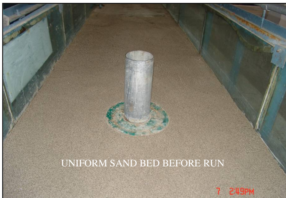
FIG.3.12 Photographic View of Collar Arrangement for the Present Study
