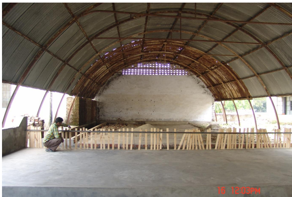
FIG. A3 Adjustable Wooden Tail Gate Provided at the Downstream End of the Flume
