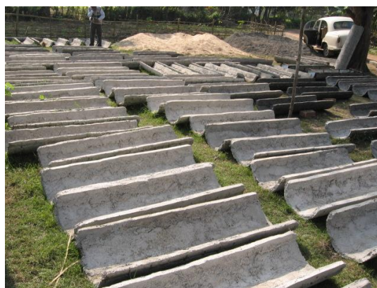
Fig.13 Bamboo-reinforced concrete section in the process of making at Atlia-Komarapur
