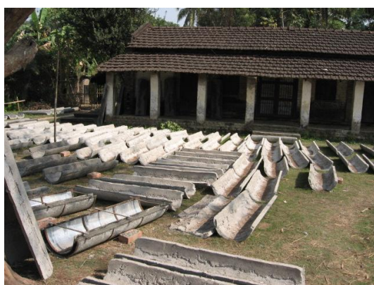
Fig.13 Bamboo-reinforced concrete section in the process of making at Atlia-Komarapur
