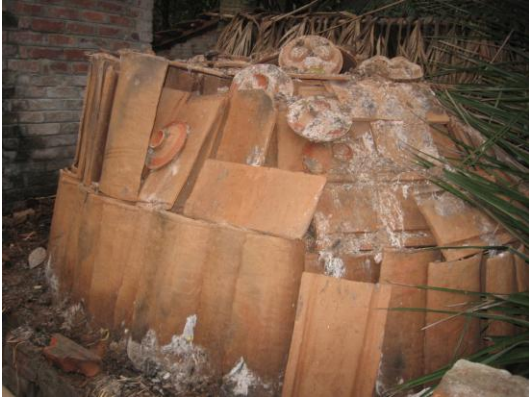
Fig.8 Tiles are burnt in indigenous kiln
