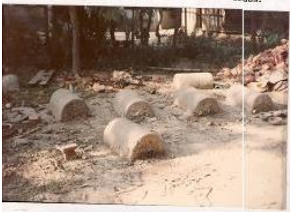
Fig. 6 Earthen mould for half round burnt clay tiles
