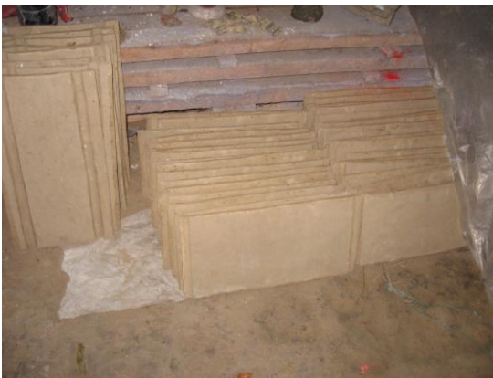
Fig.9 Air dried earthen roof tiles ready for burning
