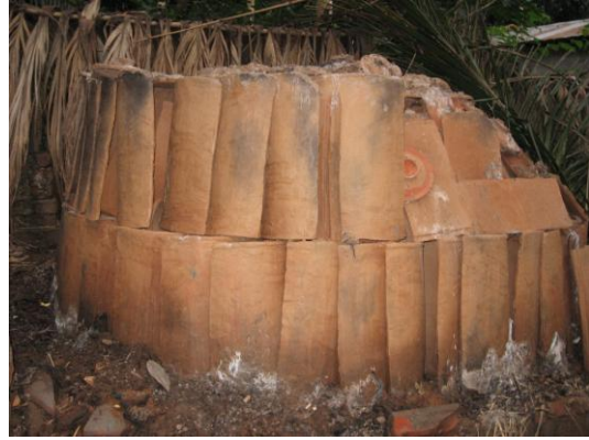
Fig.8 Tiles are burnt in indigenous kiln
