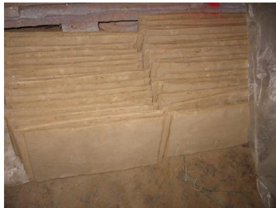
Fig.9 Air dried earthen roof tiles ready for burning
