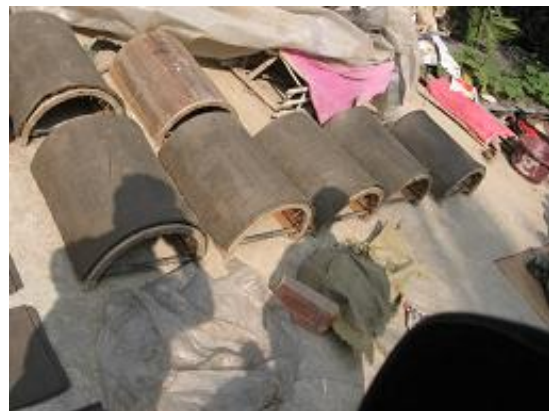
Fig. 7 Wooden mould for half round burnt clay tiles
